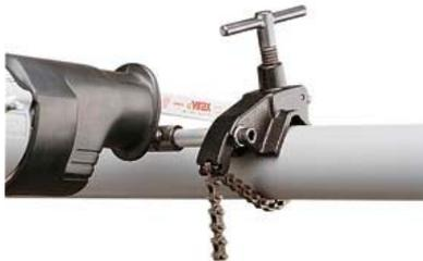
**Capacity: 4''.** Fits all shapes . For making square-cuts in pipes and sections.
